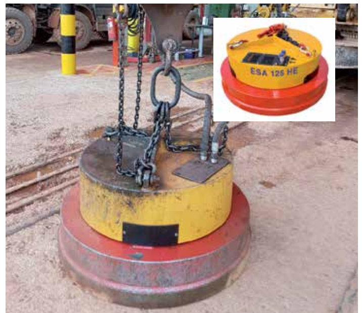
Hydraulic lift magnet purpose built for Kinross Chirano in Ghana
