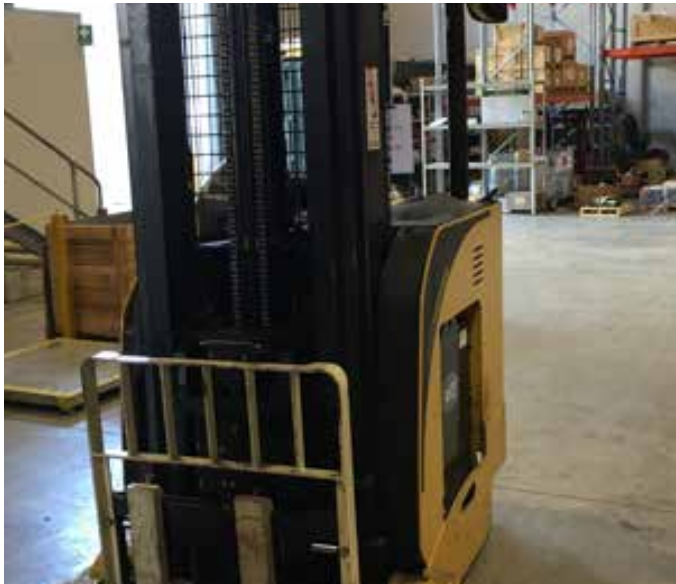
The Electric High-Reach Forklift used at WCS, Richlands (driver stands behind the mast)
