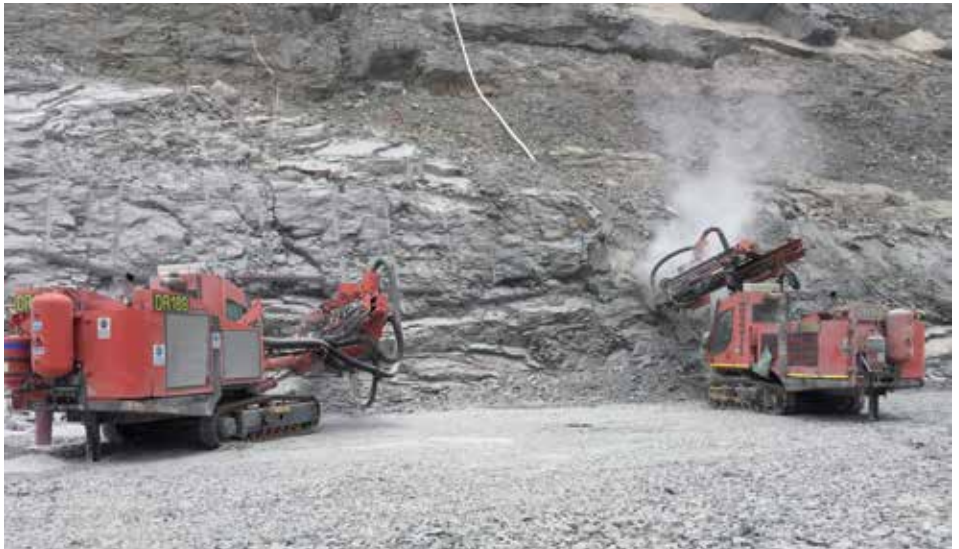
The Geotechnical Team drilling cable bolt holes at a long-term project in the Goldfields
