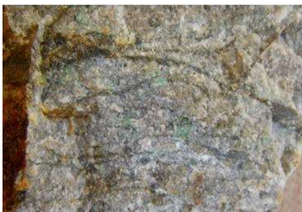
Photos 2 & 3 – Porphyry-hosted chalcopyrite mineralisation in veinlets (with magnetite and pyrite) and malachite staining in a hand specimen (left) and magnified (right).
