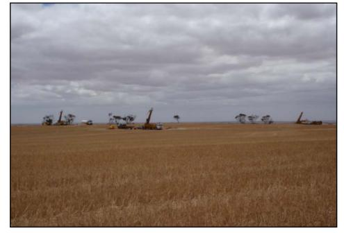
Figure 2 – Drilling at the Warramboo Project is being undertaken by one RC drill rig (for precollars) and two diamond drilling rigs (for diamond tails).
