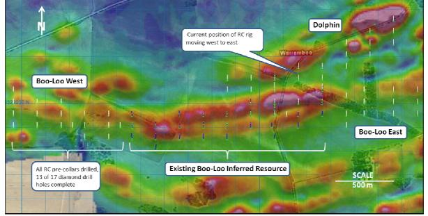
Figure 1 – Plan view of Central Eyre Iron Project highlighting Boo-Loo and Dolphin Resource expansion drilling progress. Existing holes shown in blue, current programme holes in white.
