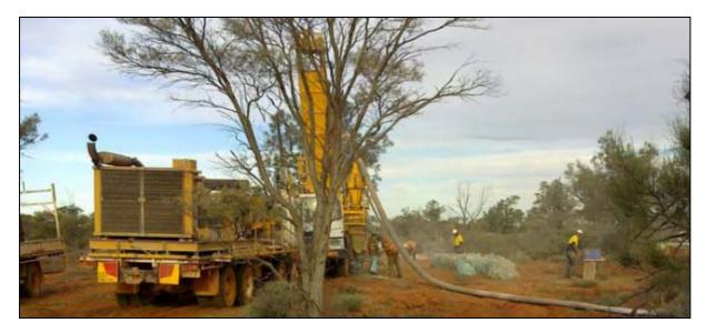
Figure 1 – Stage 1 RC drilling at the Gawler Iron Project, South Australia.
