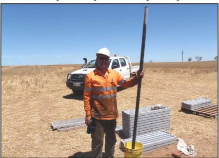
Figure 2 – Alan Rose, Coughlan Drilling, holding magnetite gneiss diamond core with typical high competency and recovery.
