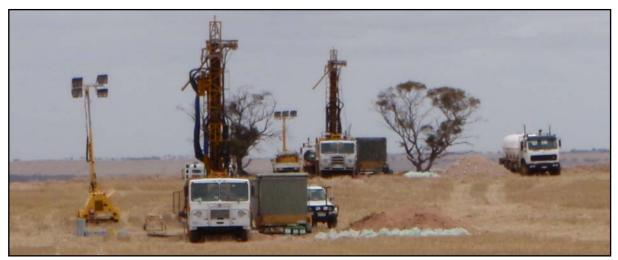
Figure 1 – Diamond drilling at Boo-Loo West, Central Eyre Iron Project.
