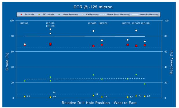
Figure 2 – Graph showing Fe grade, SiO2 grade, mass recovery and Fe recovery for samples arranged west to east across the Boo-Loo – Dolphin prospect (grind of -125µm).
