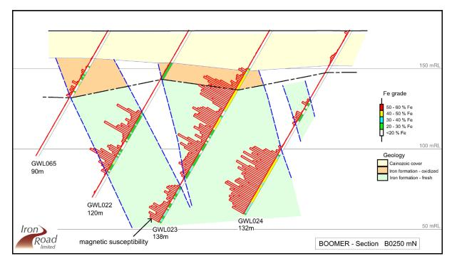
Figure 4- Cross section through Boomer showing thin hematite cap on coarse grained magnetite gneiss.
