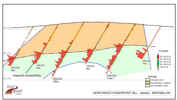
Figure 3- Cross section through NW Fingerpost Hill showing extensive hematite cap to a depth of approximately 55m.
