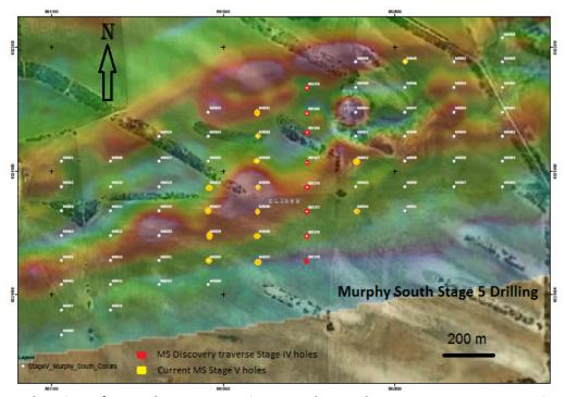
Figure 1 – Plan view of Central Eyre Iron Project Murphy South Stage 5 Resource expansion drilling progress. Existing holes shown in red, holes complete under current programme holes in yellow and holes to be drilled in white.
