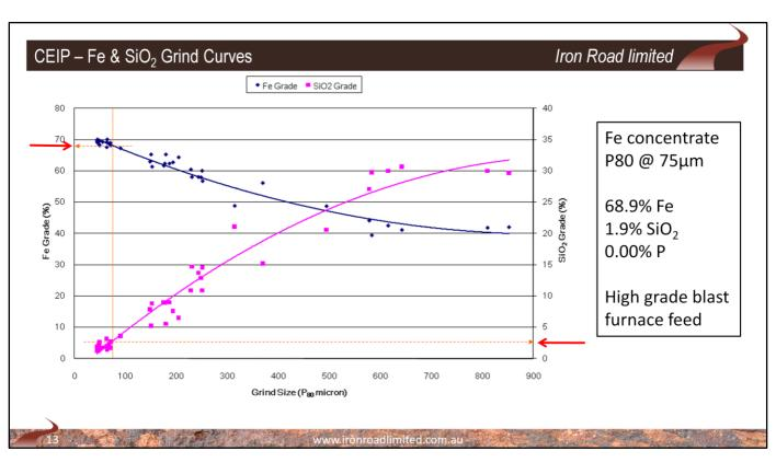
• Iron and silica curves derived from various grind sizes indicates an optimum product at 75um. This grind size is more than double than that of most WA magnetite projects where grinding as low as 28um is required
