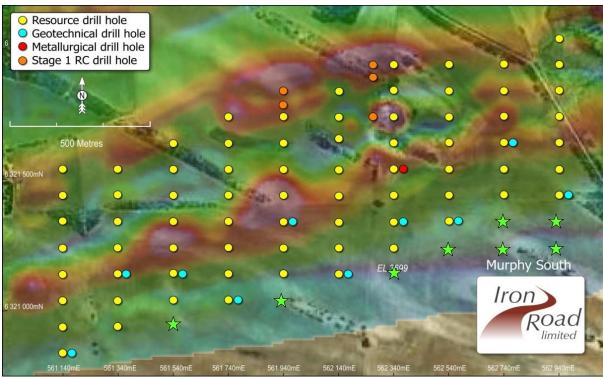
Figure 3 Plan of Murphy South – geotechnical drill hole collars shown in blue, current resource extension drill holes in green.
