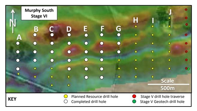
Figure 1 Plan view of Central Eyre Iron Project (CEIP) Murphy South Stage VI Resource drilling programme. Drill holes completed from current programme shown in white.
