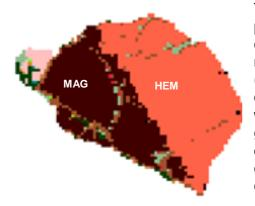
Figure 1 – Pictorial map of a -300+212µm mixed iron oxide particle in the rougher magnetic separation concentrate.
