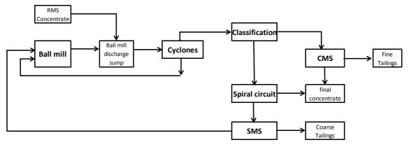
Figure 4 – Schematic block diagram of proposed spiral gravity beneficiation circuit
