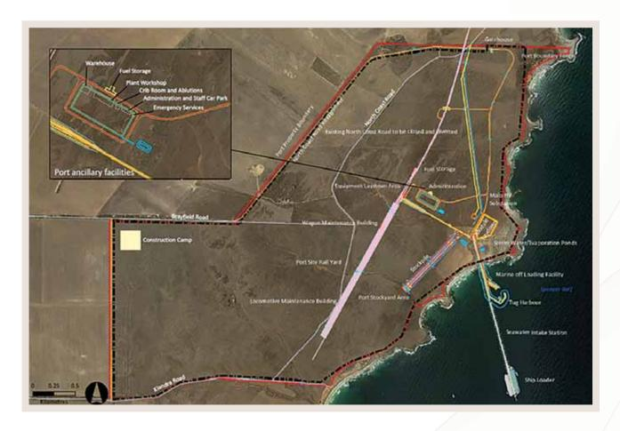
Figure 10: Current port layout at Cape Hardy including tug harbour and module offloading facilities (MOF).
