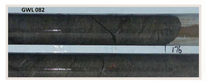
Figure 22: Typical mineralised PQ core from metallurgical drill hole GWLO82
