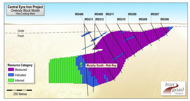
Figure 6 Cross section through Murphy South / Rob Roy (MSRR). The deeper part of the orebody is reported in the inferred category.
