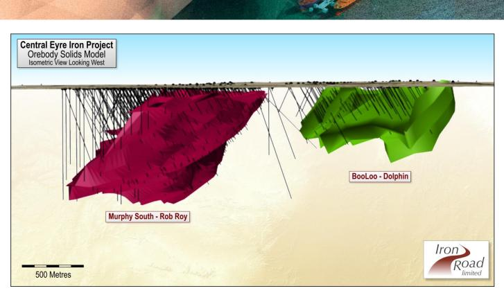
Figure 5 Cross section through Murphy South / Rob Roy (MSRR) and Boo Loo / Dolphin (BLD). The deeper parts of the MSRR orebody and the entire BLD orebody are reported in the inferred category.
