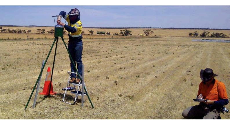
Collection from dust deposition gauge near proposed mine site at Warramboo
