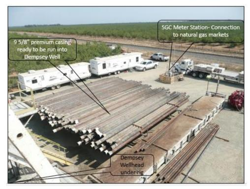
Image from Rig Floor showing Casing and Gas Meter Station
