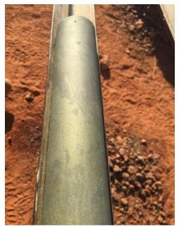
Massive sulphide mineralisation from hole TLDD0004A
