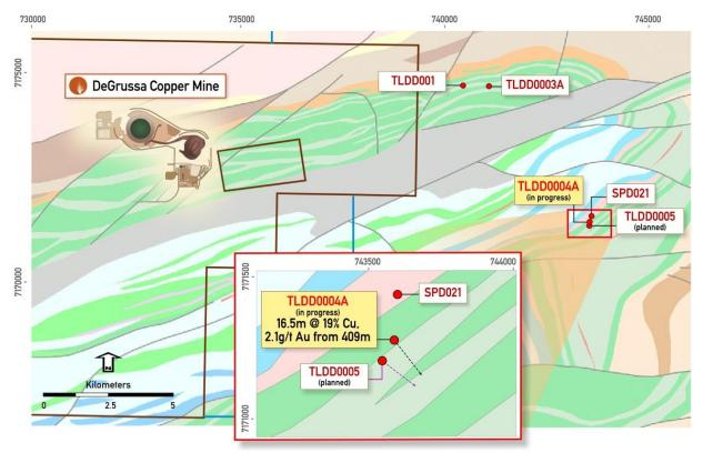
Figure 3 – Plan view showing location of recent drilling by Sandfire relative to the DeGrussa Copper Mine, including the high-grade intersection in TLDD0004A and planned step-out hole TLDD0005
