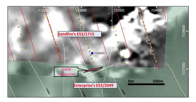
Figure 2. Doolgunna, Homestead DHEM survey status overlaid on reduced to pole, first vertical derivative magnetic image. Hole DGDD415 DHEM model in pink. Sandfire FLEM survey lines in red. Enterprise Slingram MLEM survey lines in yellow. Combined original ground EM target model in translucent white. SFR aircore drilling in yellow.
