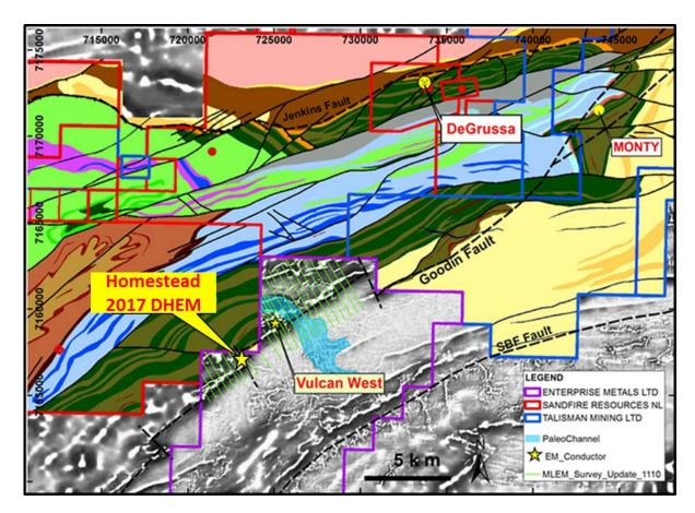
Figure 1. Plan showing off- hole DHEM conductor location and interpreted geology
