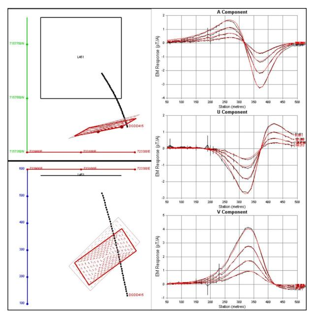
Figure 3. DGDD415 modelling of channels 32 to 35 (80–156 ms). Translucent background plate corresponds to modelling of channels 20 to 24 (6 – 14.5 ms). Black and red profiles represent field and modelled response respectively.
