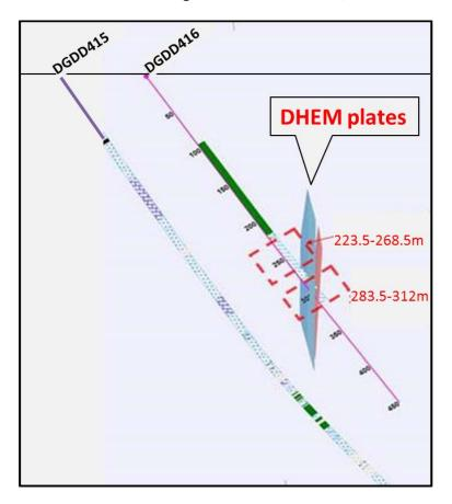
Figure 1. Schematic Section Showng DGDD415 & DGDD416, with DHEM Conductor
