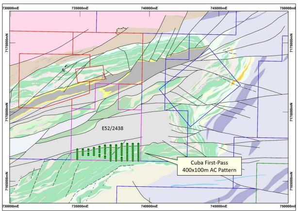
Figure.3. AC Drilling conducted at the Morck Well Project during Q1, 2019 (Auris Tenements labelled with pink outline)
