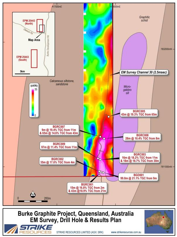
Figure 2 - EM Survey - Burke Prospect, Burke Graphite Project
