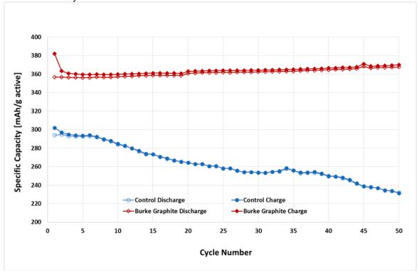
Figure 1 - Comparison of control cells and Strike's natural graphite (20 μm) showing charge and discharge capacities for 50 cycles at C/10 rate and 25 °C
