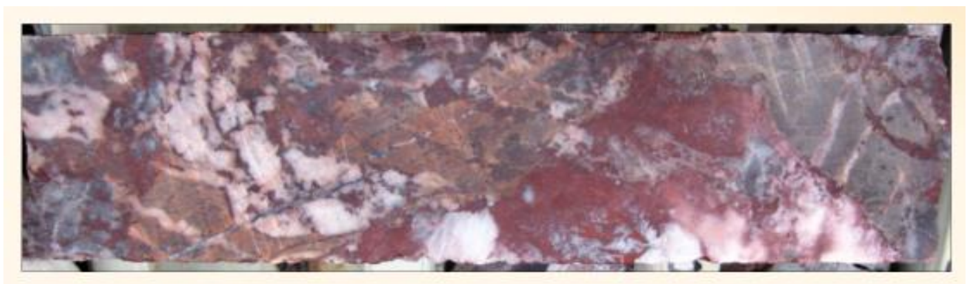
Figure 4 – Strong Hematite-K Feldspar-Silica-sulphide alteration/vein zone
