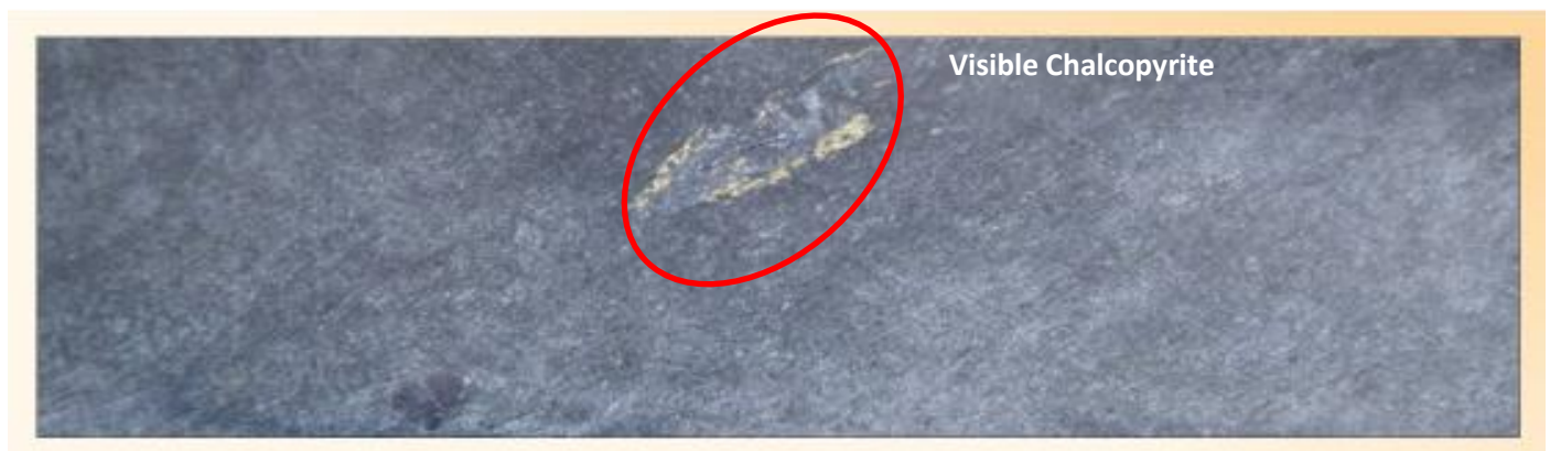
Figure 4 – Strong Hematite-K Feldspar-Silica-sulphide alteration/vein zone
