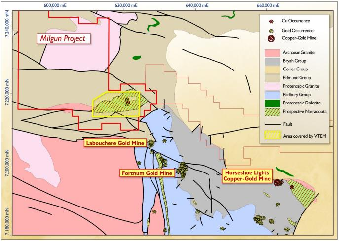
Figure 3 – Milgun Project geology showing copper/gold occurrences, distribution of prospective Narracoota Formation and area covered by VTEM survey
