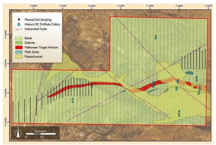
Figure 2: Soil sampling grid over western extension of the Halloween VMS-target horizon and to test a malachite-bearing sedimentary unit to the north-east of the main trend.
