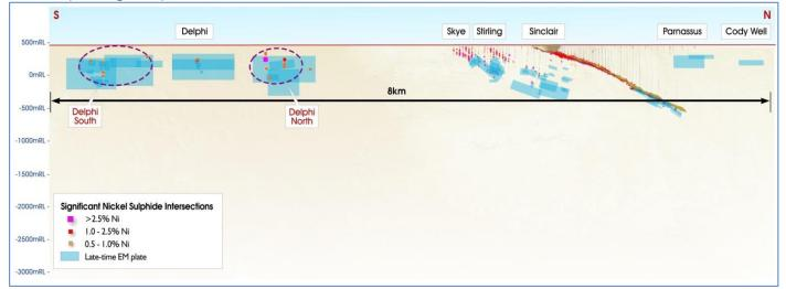
Figure 2: Sinclair Trend longitudinal projection showing 8km of strike extent, late-time EM plates and historical mineralised intercepts.
