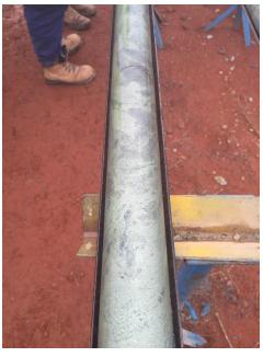
Massive sulphides with visible chalcopyrite in diamond drill core from hole TLDD0005
