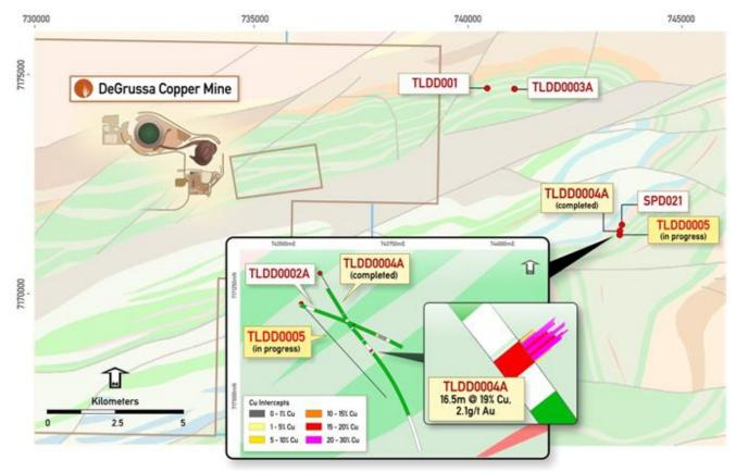
Figure 2 – Plan view showing location of recent exploration drilling relative to the DeGrussa Copper Mine, including the high-grade intersection in TLDD0004A and step-out hole TLDD0005.
