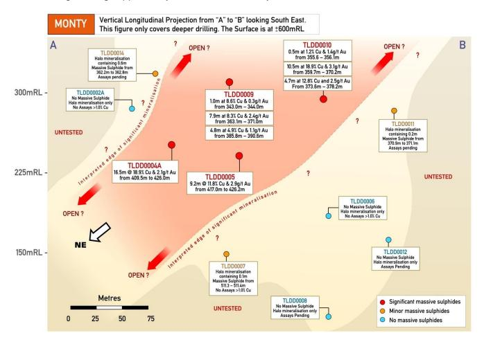
Figure 2 – Vertical longitudinal projection of Monty showing deeper drill-hole piercepoints.
