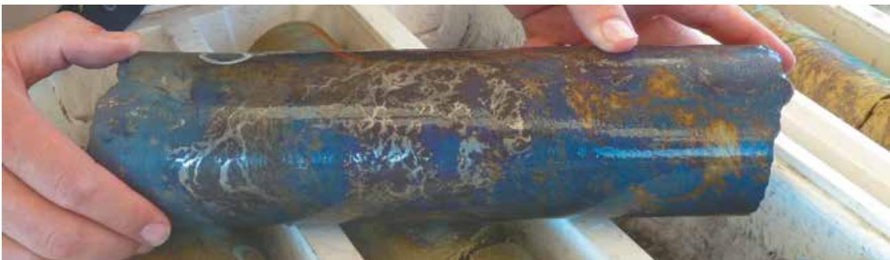
Figure 5: Large diameter (PO) metallurgical drill core from Monty Copper-Gold deposit.
