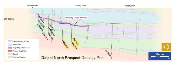
Figure 3: Delphi North drill collar plan showing recent and historic collar locations, simplified geology and Priority Target position
