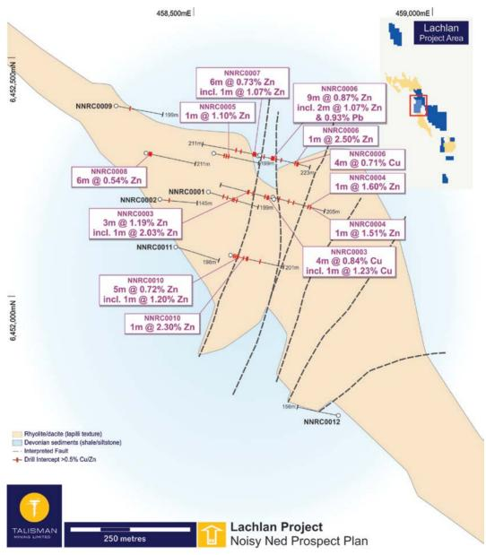
Figure 3: Noisy Ned - Drill collar locations over simplified solid geology.
