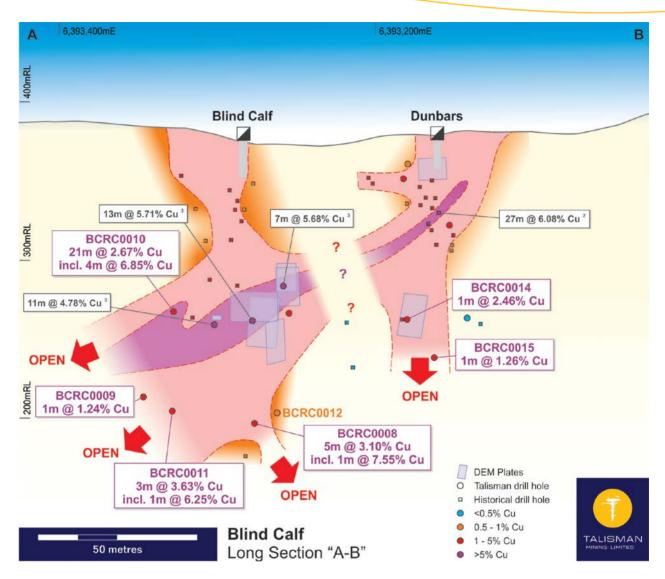
Figure 1: Blind Calf Prospect - long section showing Blind Calf-Dunbars lode recent and selected historical drilling results<sup>2</sup>.
