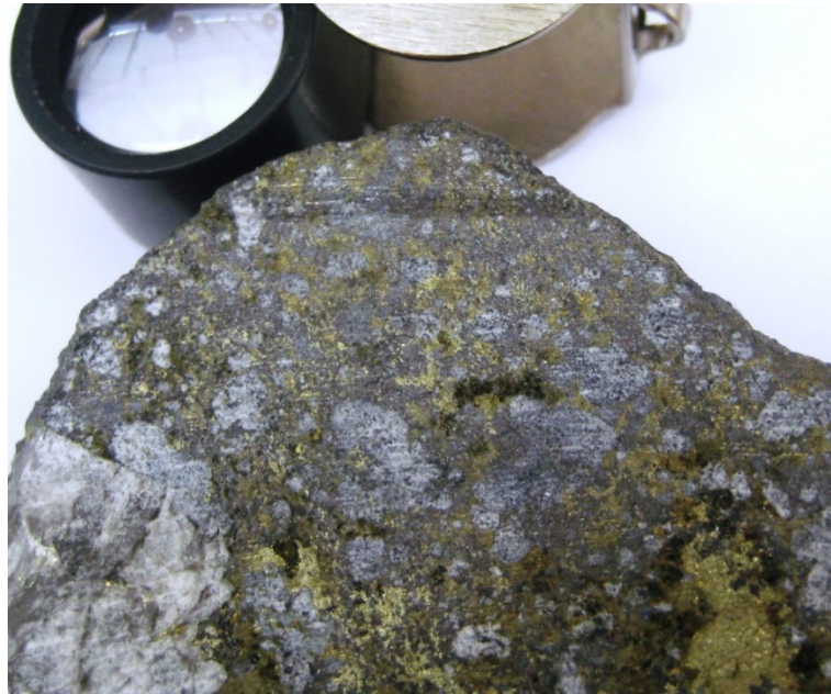
Figure 3 – Browns Prospect: Section of core from hole 13MHDDH015 at 78.1m, showing copper in chalcopyrite (shiny yellow), lead in galena (shiny silver flecks), and zinc in sphalerite (dark grey zones). The hand lens shown for scale is 18mm wide.
