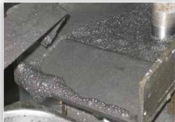
↑ Figure 2. TOP - Cumulative Recovery over Duration of Flotation Test (METS data), and BOTTOM - First pass flotation concentrate photograph.
