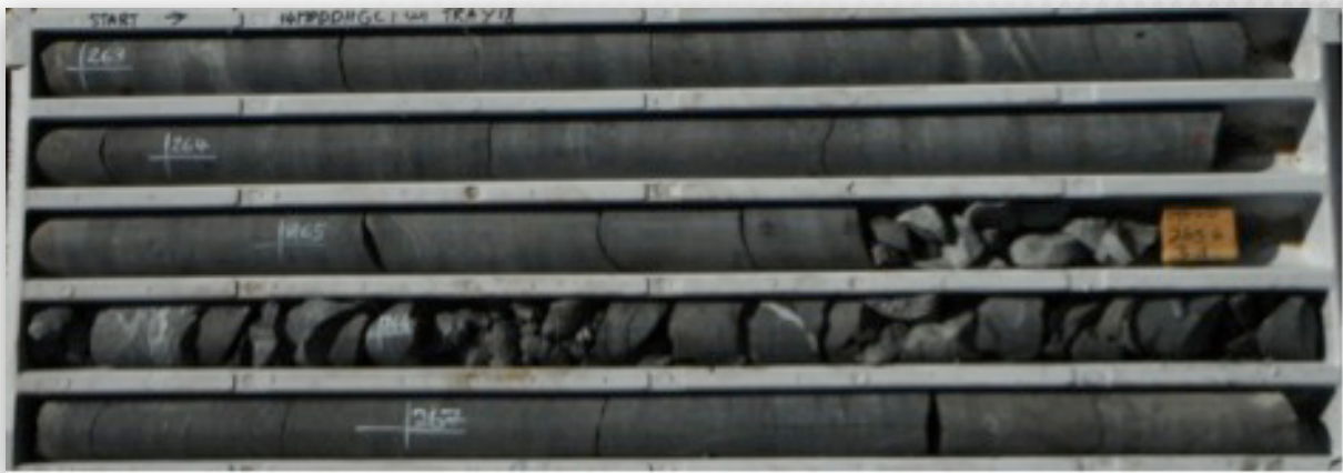
↑ Figure 1: Core tray #18 from 14MPDDHBGC1W1 from 262.95 to 267.65m, showing typical dark grey graphitic core.
