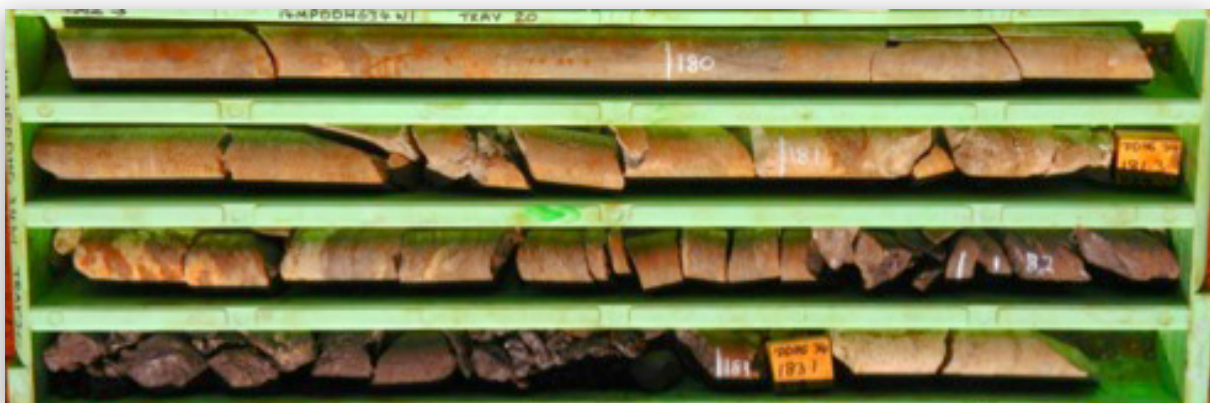
↑ Figure 2: Core tray #20 from 14MPDDHG34W1 from 179.4 to 183.3m, showing the pale sericite alteration and the graphite vein (from 181.8 to 183.0m).
