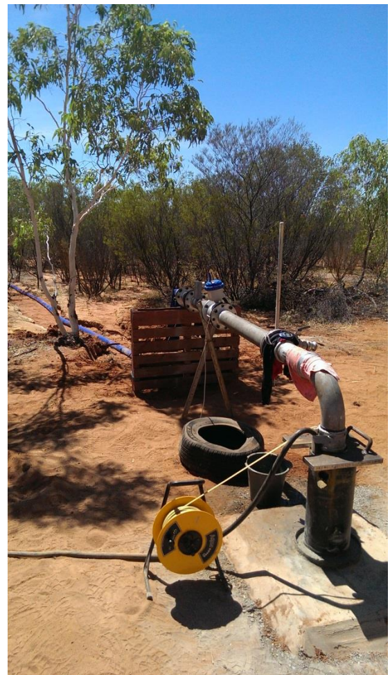
Figure 3 (Right). Pump testing on the production bore 15MPWB005, using a submersible variable pump and digital flow metering.
