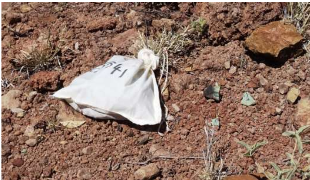
Plate 2. Detailed photograph showing the some of the shale material sampled (MC15541). Note the rubby nature of the outcrop and the green (malachite) and black (chalcocite) fragments of copper mineralisation.
