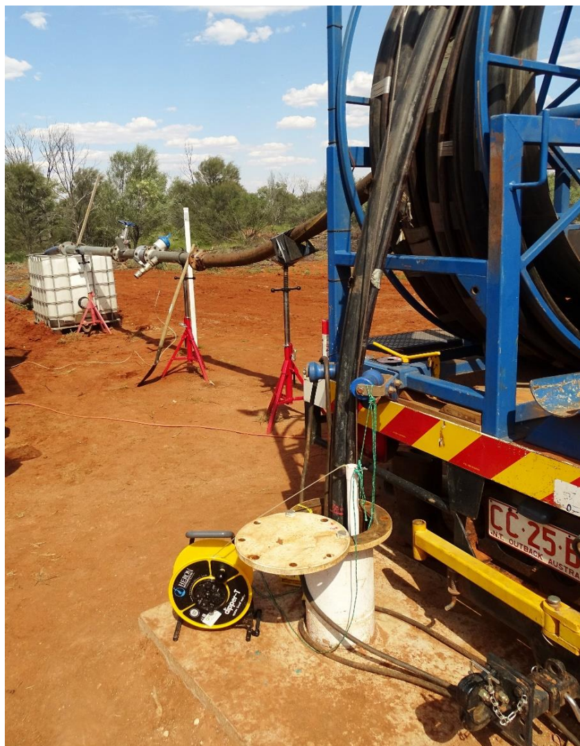
Figure 3. Measuring draw-down during the 48-hour Constant Rate pump test on hole 16MPWB015.
