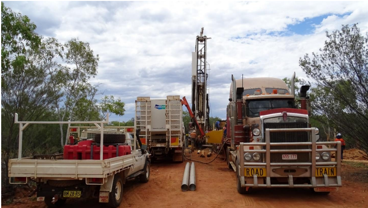
Figure 2. Running in casing, hole 16MPWB017.
