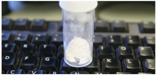
TNG's Pure white high purity Titanium dioxide prior to coating and finishing
