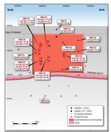
Figure 1: Interpreted Long Section of Sunrise mineralisation showing recent intercepts.
