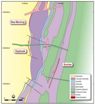
Figure 2: Geological plan showing Sunrise and New Morning mineralisation.
