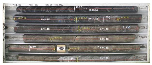
Figure 1: Mineralised drill core from NMD 177 showing high grade massive nickel sulphides
