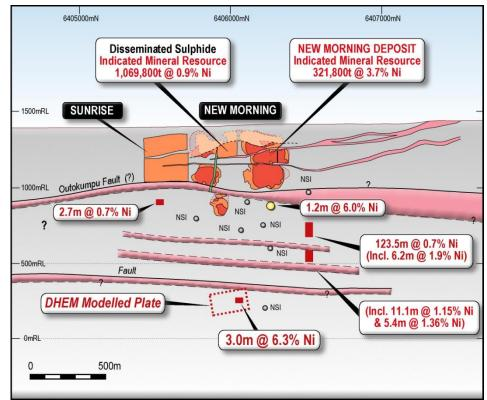
Figure 2, New Morning Long Section showing NMD177 and interpreted DHEM plate
