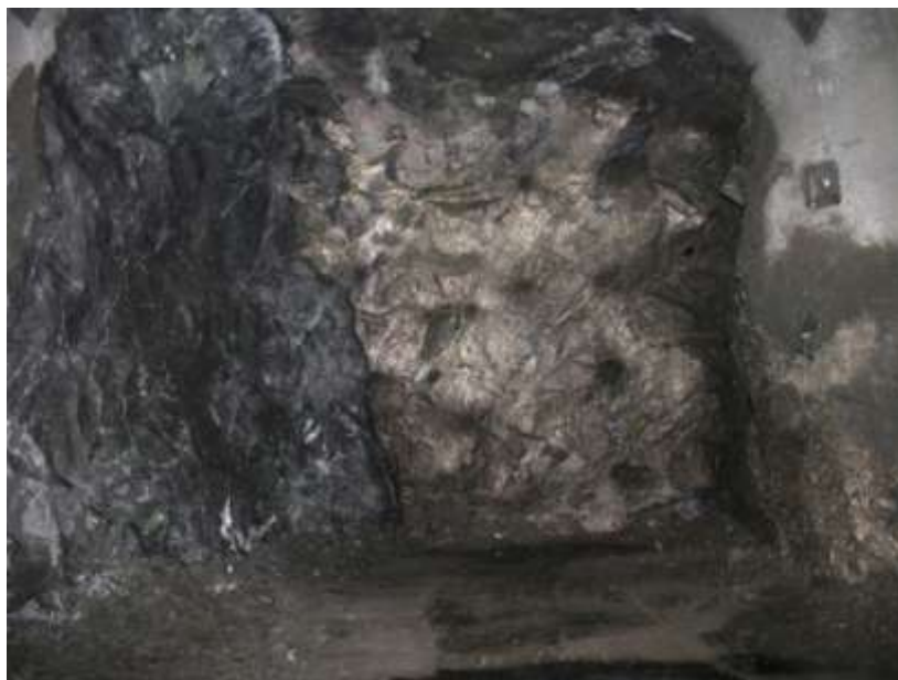
295 SOD ore drive showing face of massive sulphide (Face grade 5% Ni)
