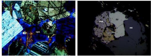
Figure 9: Petrology micrographs of olivine gabbronorite (left) and secondary pyrite after pyrrhotite, violarite after pentlandite and chalcopyrite (right) in drill hole WGA0008. Fields of view are 2.4mm (left) and 225 microns (right)
