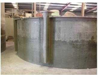
FRP leach tank top section during manufacture
