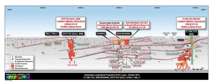
Figure 4: Interpreted long projection of the Western Belt footwall contact extending from south of Spotted Quoll to Flying Fox, showing new and planned drilling
