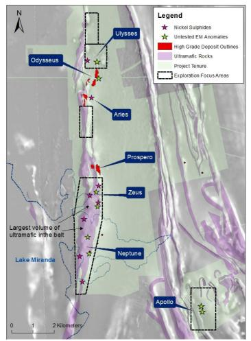
Figure 6: Cosmos Nickel Complex – Exploration focus areas and known locations of existing EM and nickel anomalism (overlaying Mag 1VD)
