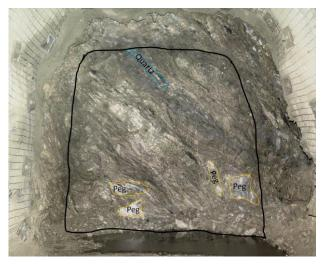
385 SOD ore drive with a face grade of 7.3% Ni
