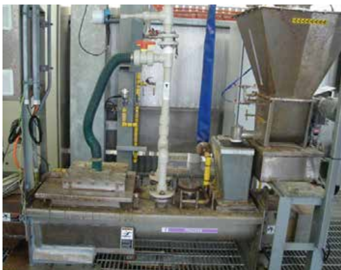
▼ Figure 5.5: Acid-Concentrate Mixer, External (above) and Internal (below)
