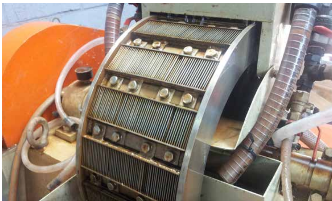
▼ Figure 5.2: Magnetic Separation using WHGMS 500
