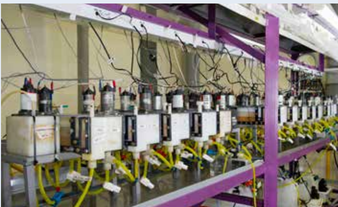
▼ Figure 5.8: SX Circuit for Production of Separated REOs
