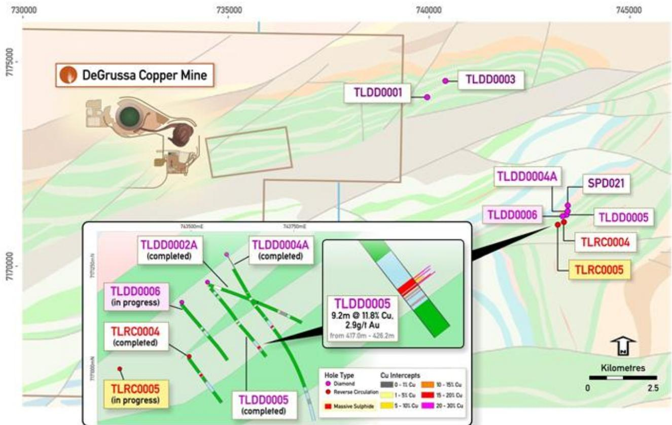
Figure 2 – Plan view showing location of recent exploration drilling relative to the DeGrussa Copper Mine, including recent and current diamond and RC drilling and the newly reported assay results for TLDD0005.
