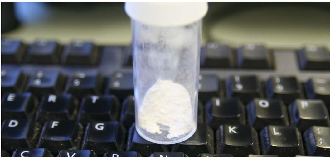
TNG's Pure white high purity Titanium dioxide prior to coating and finishing
