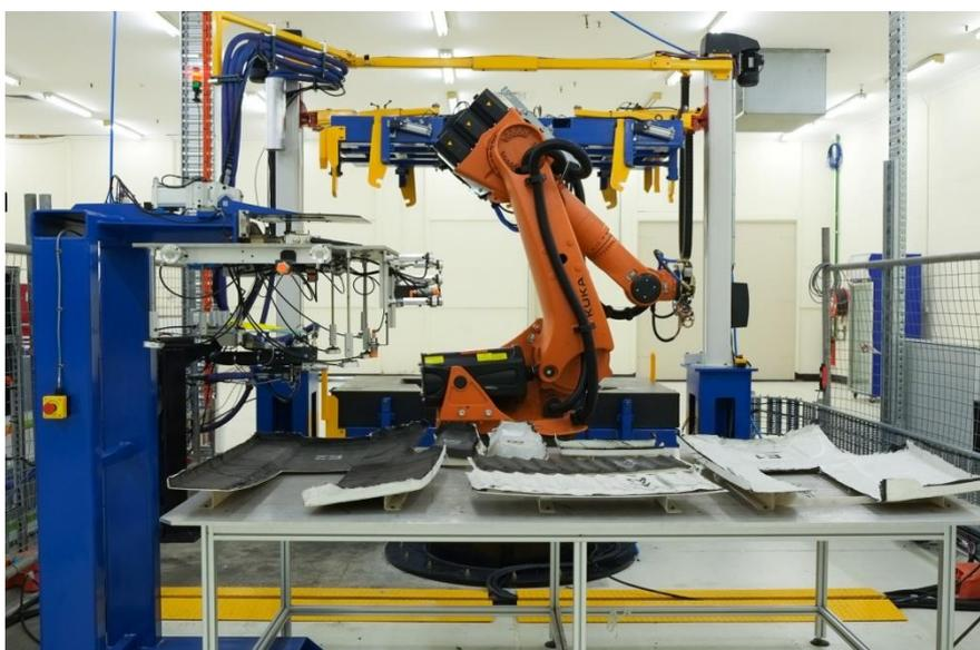
Quickstep’s resin spray transfer (RST) technology automates production of strong, lightweight carbon-fibre composite car panels
