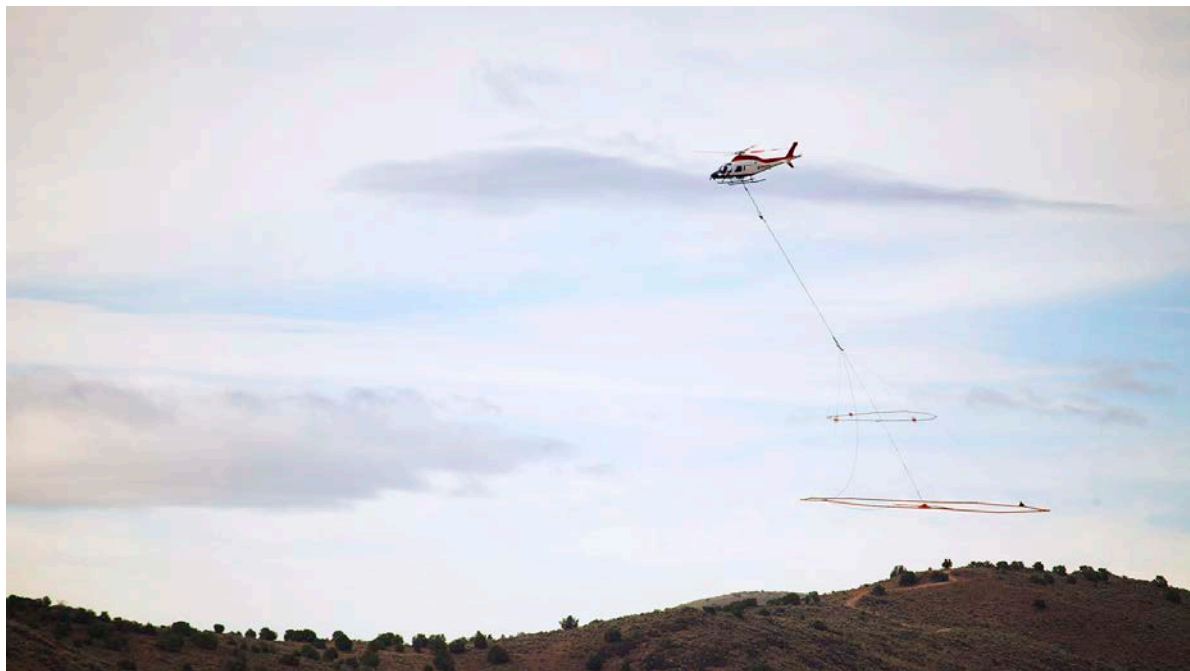
Figure 1: Helicopter-borne Versatile Time-Domain Electromagnetic (VTEM™ Max) geophysical system
